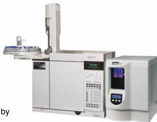
H2PEM Hydrogen Generator with Agilent 7890 GC-FID
